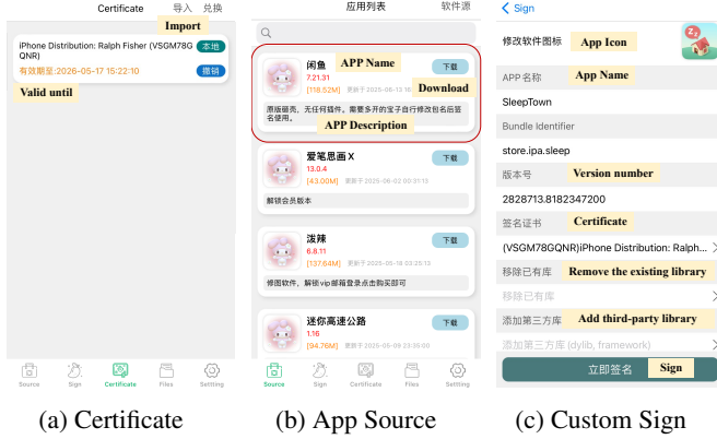
Figure 8: Core features of a typical signing tool.
